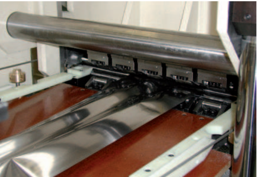
Extrem welliger Edelstahl im Richtmaschineneinlauf Extremely deformed stainless steel in front of the leveler
