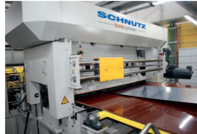
Multi-Blanking-Anlage für Edelstahl Multi-Blanking-Line for Stainless Steel
